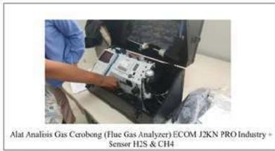
Alat Analisis Gas Ccrobong (Flue Gas Analyzer) ECOM J2KN PRO Industry -
